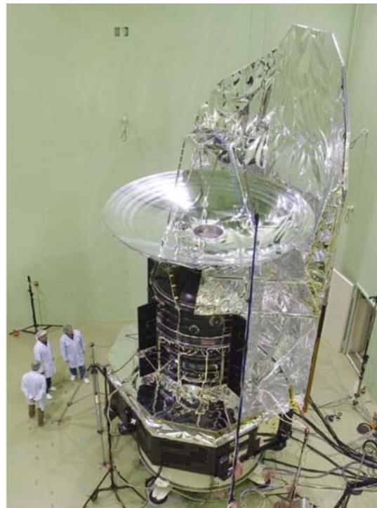
**Fig. 1** The *Herschel* Space Observatory shown in a clean room before launch.
